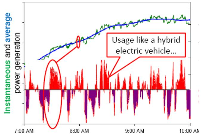
Fig. 3, Conceptual illustration of varying power output for Frequency Regulation cycling around an average plant power output value
