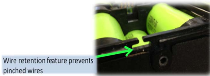
Figure 5 ALM 12V35 Mechanical Design, Wire Retention
