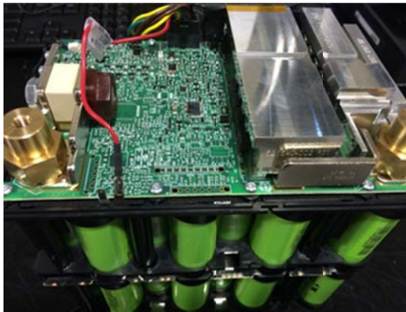
Figure 2 ALM 12V35 Cell Management Protection Circuitry
