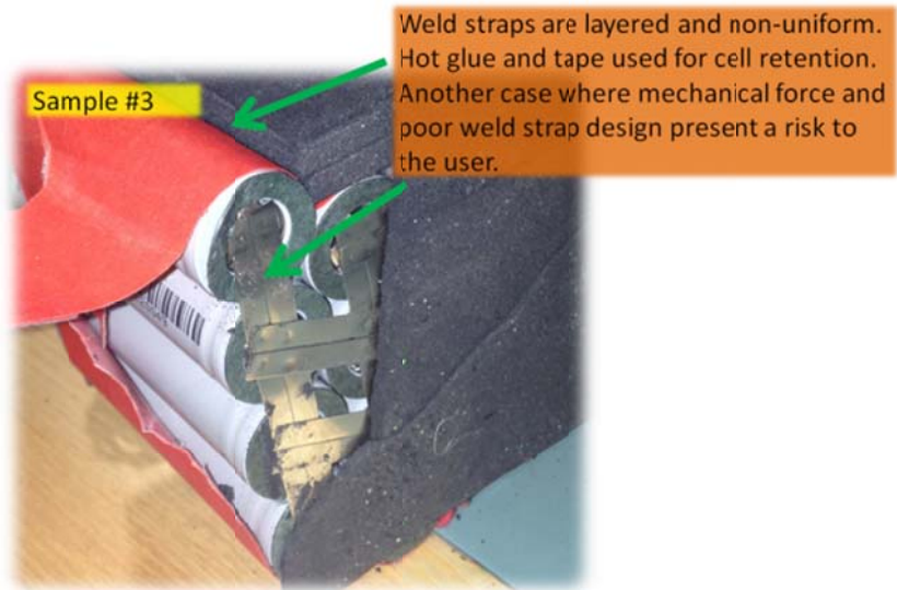
Figure 8 Sample #3 Non-uniform Weld Strap Design Present Risk to the User
