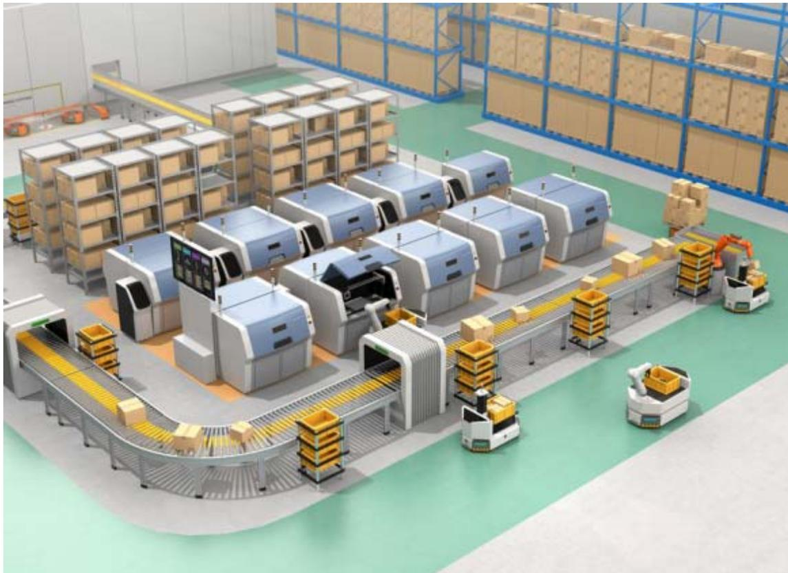
Battery-operated Automatic Guided Vehicles, or AGVs, are quickly becoming an appealing option in manufacturing, warehousing and distribution across a myriad of industries. AGVs can speed up the workflow by handling tasks such as moving raw materials, pallets and finished products, and loading and unloading trailers and containers.
